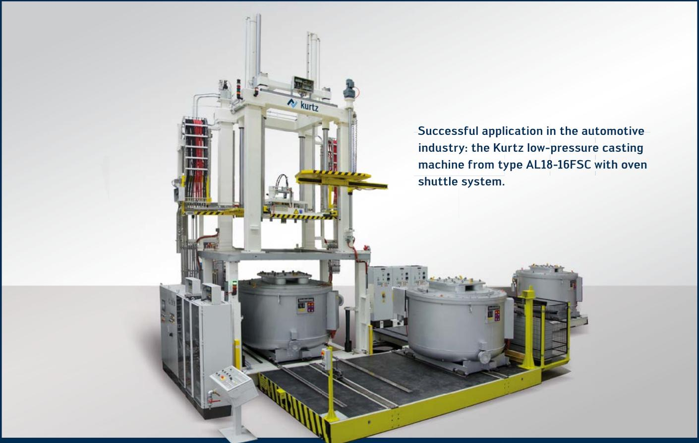
Successful application in the automotive industry: the Kurtz low-pressure casting machine from type AL18-16FSC with oven shuttle system.
